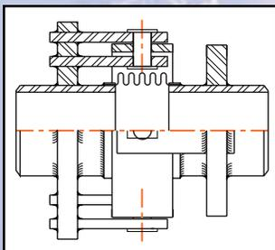
This expansion joint contains a single bellows element and is designed to permit angular rotation in any plane, by utilizing two pairs of hinges connected to a common central floating ring or box. The Gimbal Expansion Joint provides the same restraint to axial deflection and pressure thrust as the Hinged Expansion Joint. This expansion joint functions in much the same fashion
