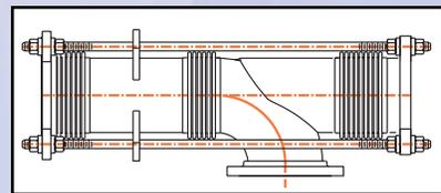
This expansion joint is a unique design that not only restrains the pressure thrust, but also balances this thrust force so that main anchoring of the
