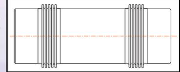
This expansion joint contains two bellows elements separated by a center pipe section or spool. This type of arrangement provides a design that
