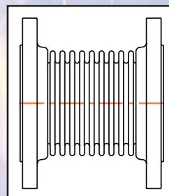
This is the simplest expansion joint available and consists of a single bellows element and end connections. This expansion joint will deflect in any mode listed under **Bellows Deflections**, and is usually the first considered in system design. The Single Unrestrained Expansion Joint will require the most control of the adjacent piping with respect to anchors and guiding. The Single Unrestrained Expansion Joint will not control the movement of the
