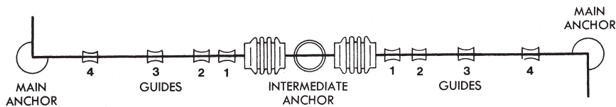
DIAGRAM #2 Two Expansion Joints in longer pipe run than that shown in Diagram #1. Intermediate anchor between main anchors forms individual expanding and contracting sections. Expansion Joints are installed between intermediate and main anchors.
