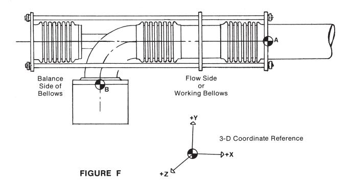
Because of the design, the Pressure Balanced Expansion Joint eliminates pressure thrust loads on mating equipment and simplifies critical piping arrangements.
