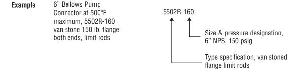
To add an optional flow liner, add an "L" to the type specification i.e. 5501RL or 5502RL
