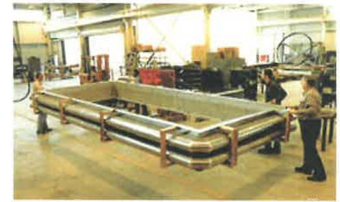
Rectangular Expansion Joint with "U" profile and double miter corners.
